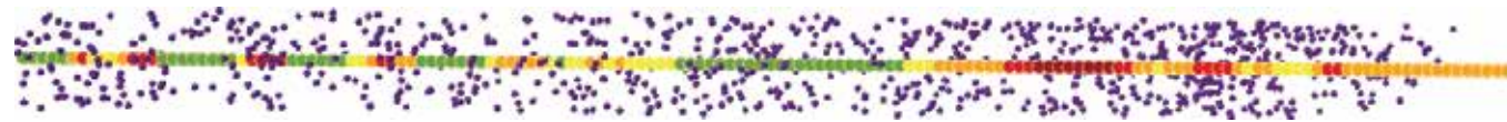
Top view of a slice of points shown in purple, and the resultant fence presented as a colored line in the center of the input points.
